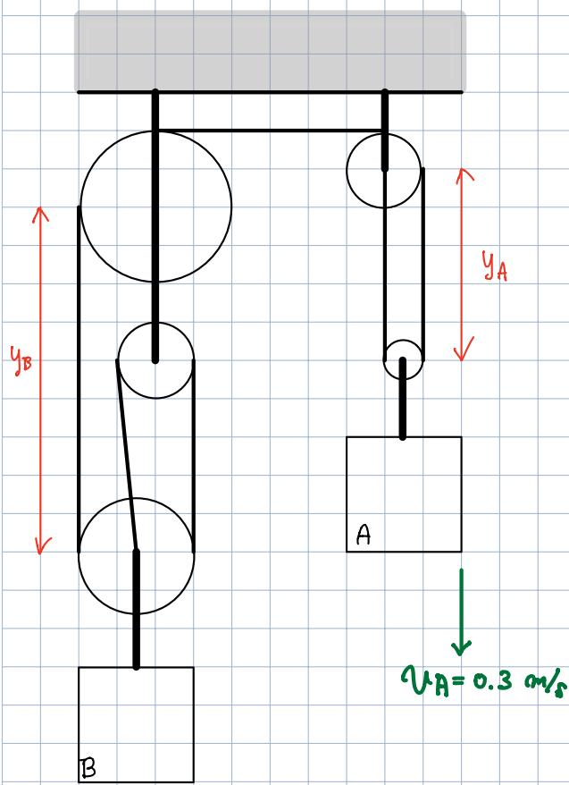
A has a downward velocity of  $0.3 \text{ m/s}$
