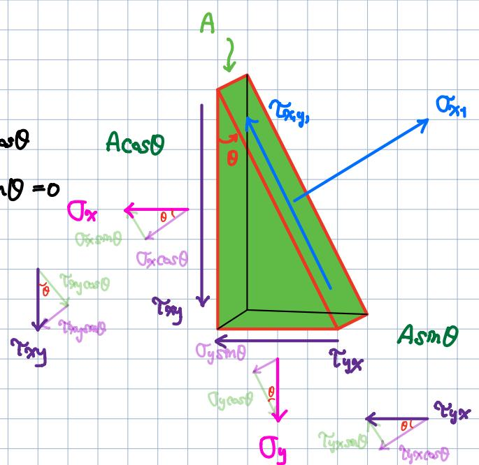
$$T_{x_1} = \frac{T_x + T_y}{2} + \frac{T_x - T_y}{2} \cos 2\theta + T_{xy} \sin 2\theta$$
